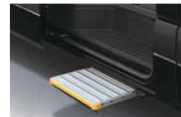
Mid-door electrical step
